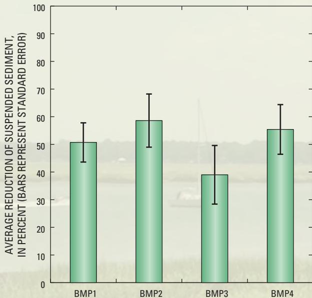
**Average reduction of suspended sediment concentration, in percent, between inlet and outlet waters of each BMP for the sampled storm events.**
