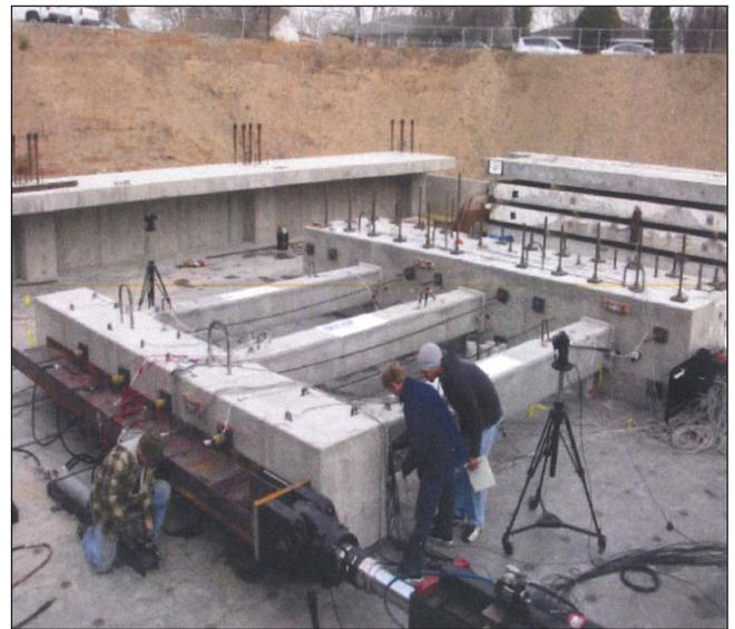
*Three-Pile Specimen Testing*
