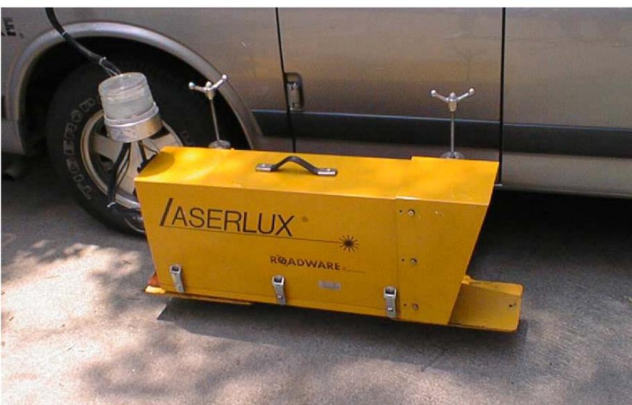
**Laserlux Retroreflectometer Attached to Van**
