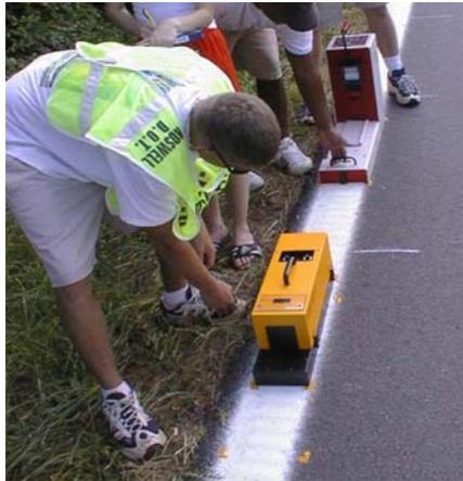
**Using Reflectometers on a Test Section**
