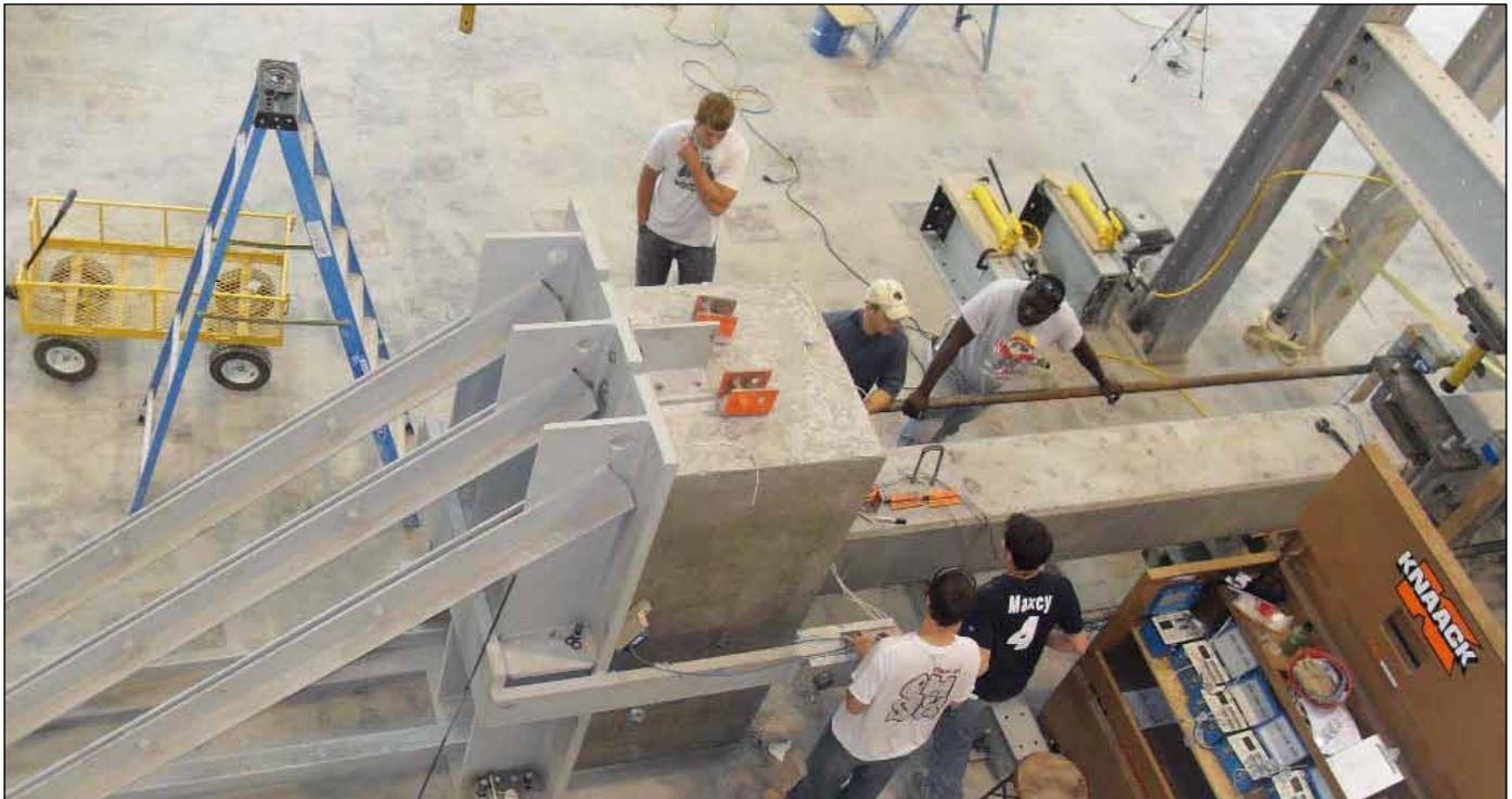
*Setup for Testing the Second Interior Pile Specimen*
