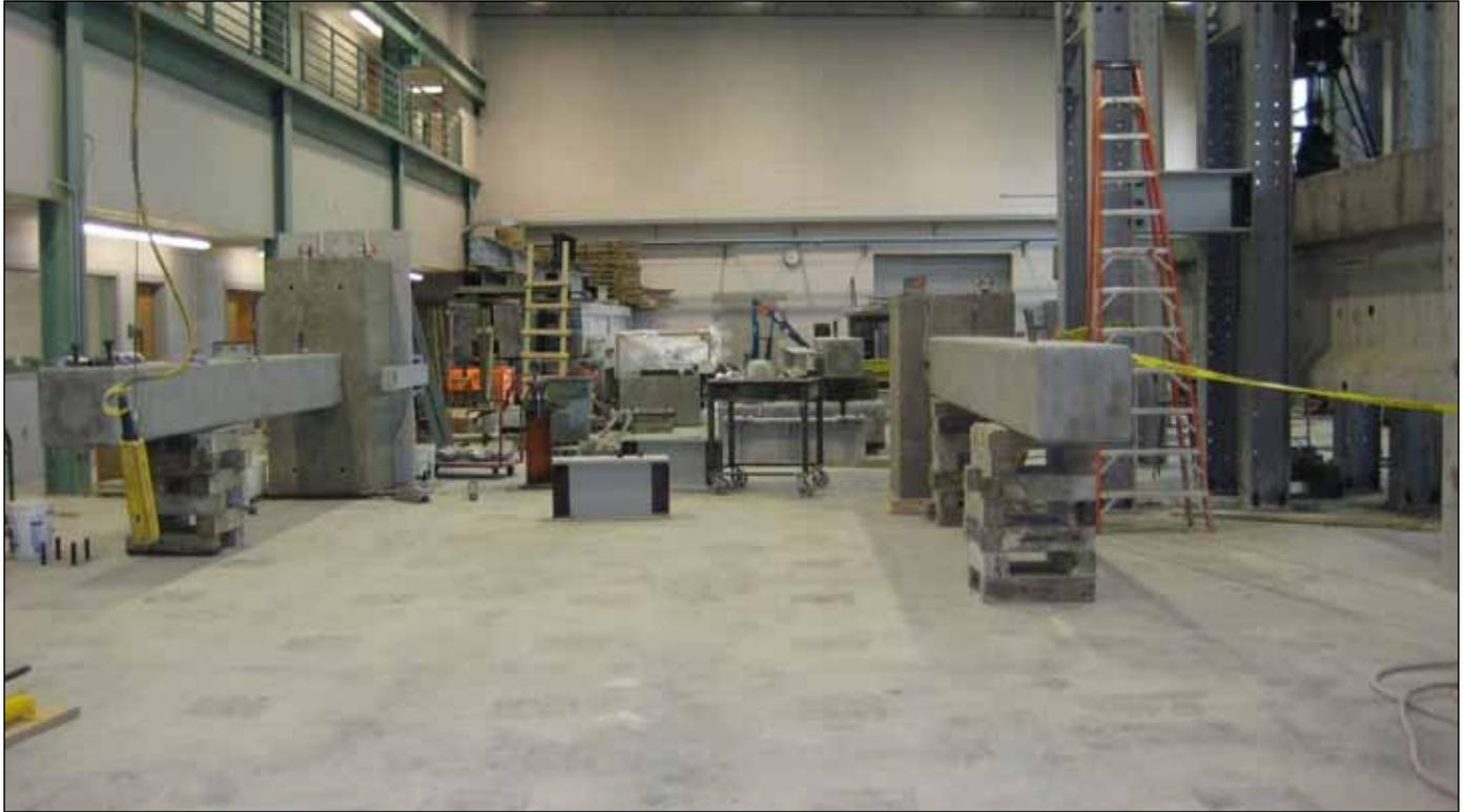
*Test Specimens with an Interior Pile on the Left and an Exterior Pile on the Right*
