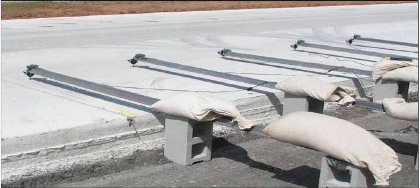
*Dial gauges used to measure elevation changes along a slab on I-385.*
