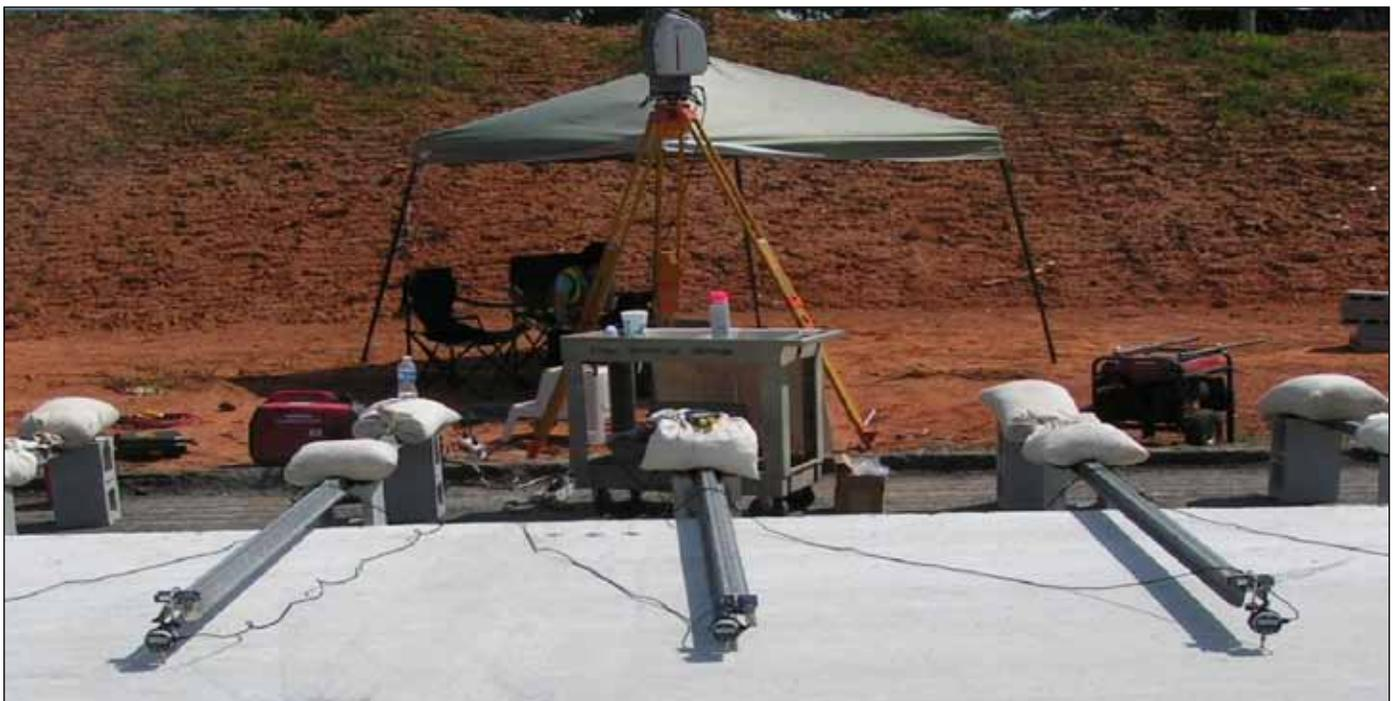
*Terrestrial laser scanner on tripod behind the dial gauges.*
