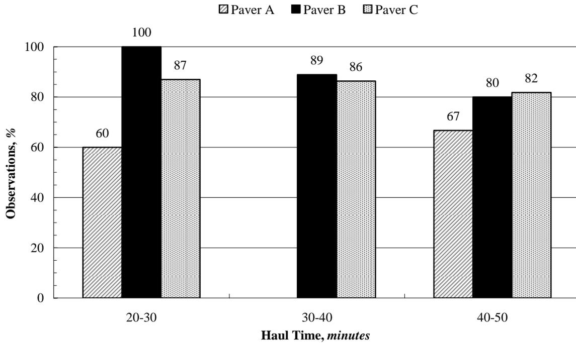
Figure B-5: TDD observations greater than two standard deviations from the mean located behind a paver.
