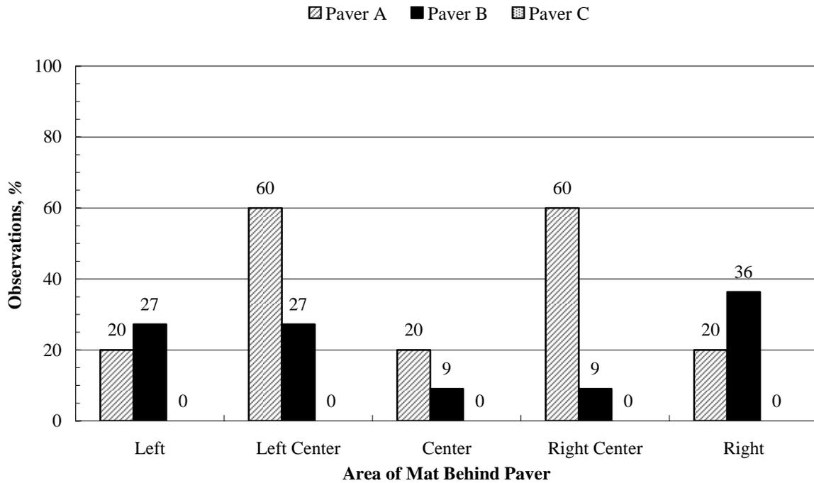
Figure B-11: TDD observations greater than two standard deviations from the mean in different locations behind the paver (40–50 min. haul time).
