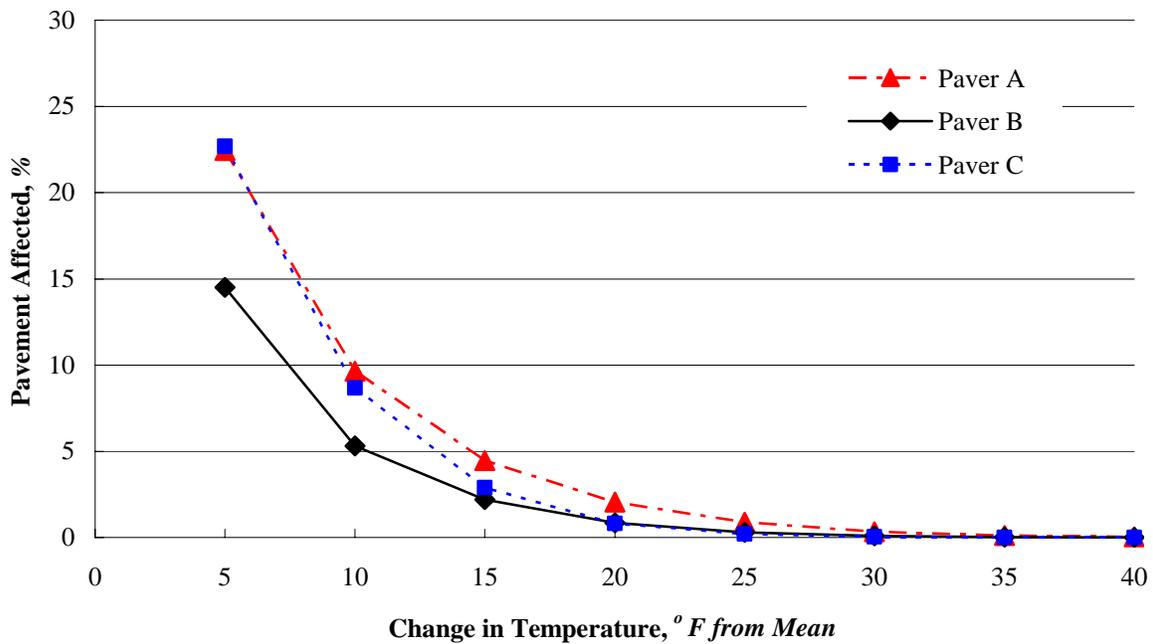
Figure 11: Comparison of TDD from different asphalt pavers from different manufacturers (40–50 min. haul time, all projects).
