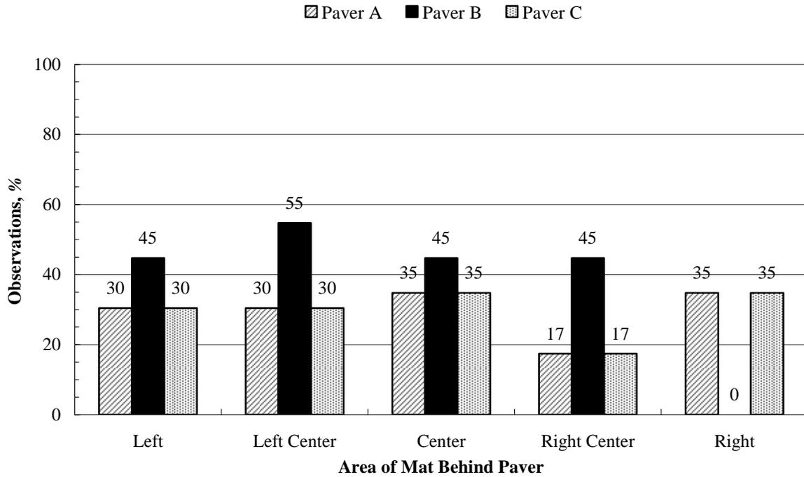
Figure B-7: TDD observations greater than two standard deviations from the mean in different locations behind the paver (20–30 min. haul time).
