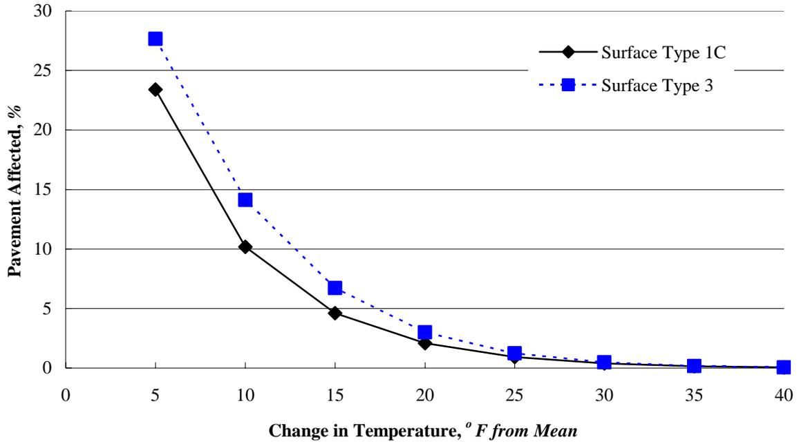
Figure 20: Effect of mix type on TDD (20–30 min. haul time).
