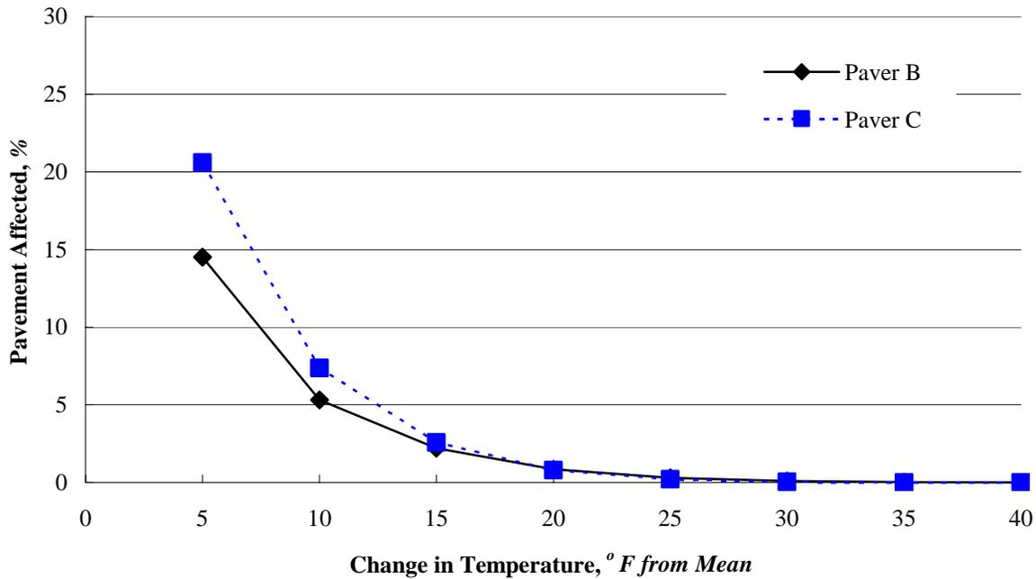
Figure B-2: Comparison of TDD from different asphalt pavers from different manufacturers (40–50 min. haul time, daytime paving).
