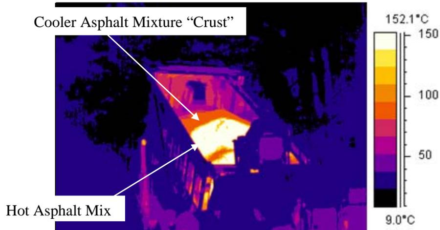
Figure 2: Temperature variations in haul truck.
