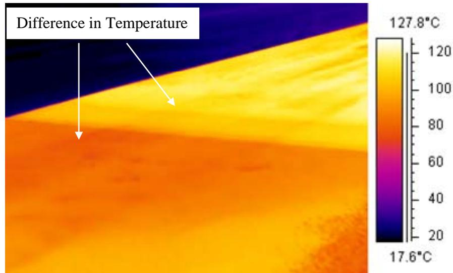
Figure 4: Difference in temperature due to paving delay.
