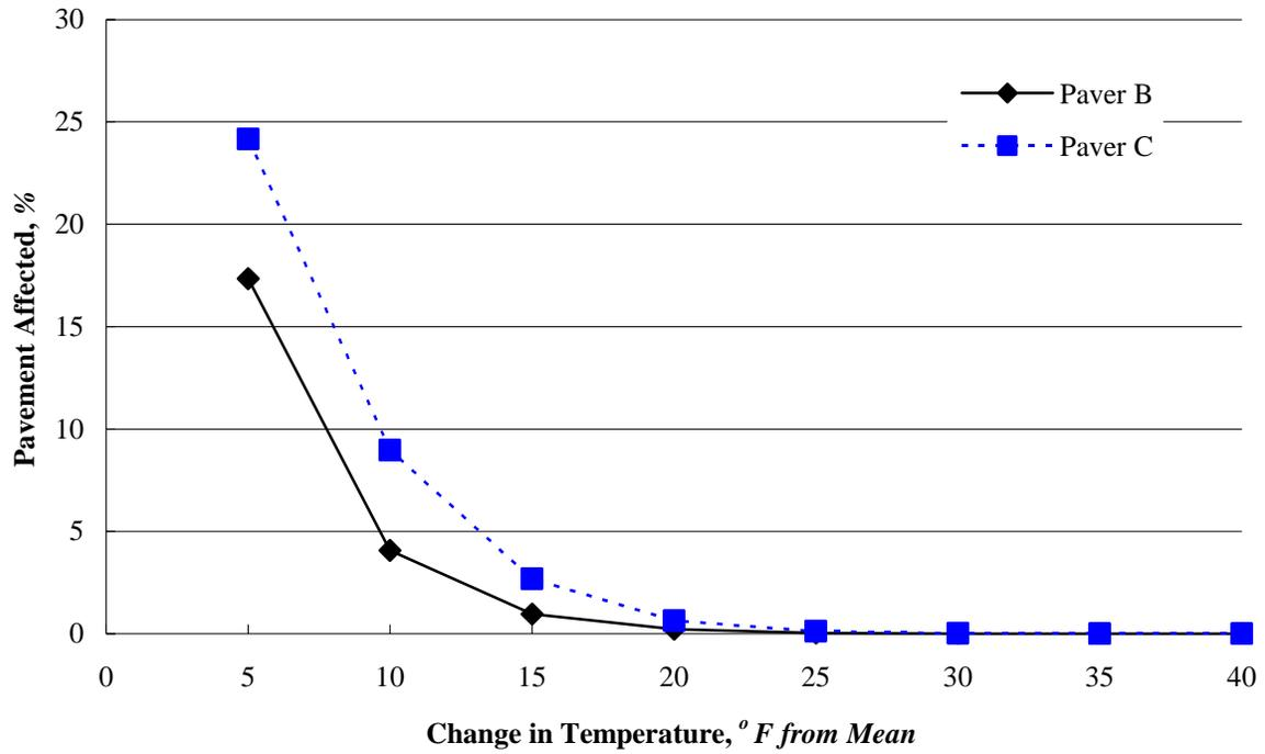
Figure 10: Comparison of TDD from different asphalt pavers from different manufacturers (20–30 min. haul time).
