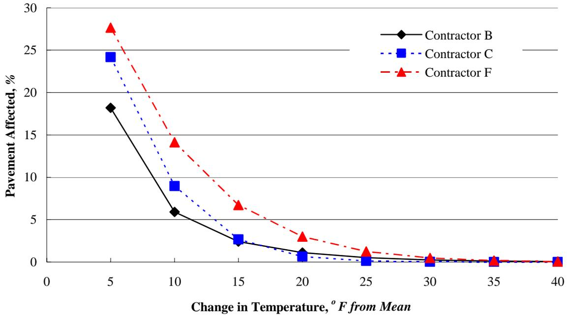
Figure 22: Effect of contractor on TDD (20–30 min. haul time).
