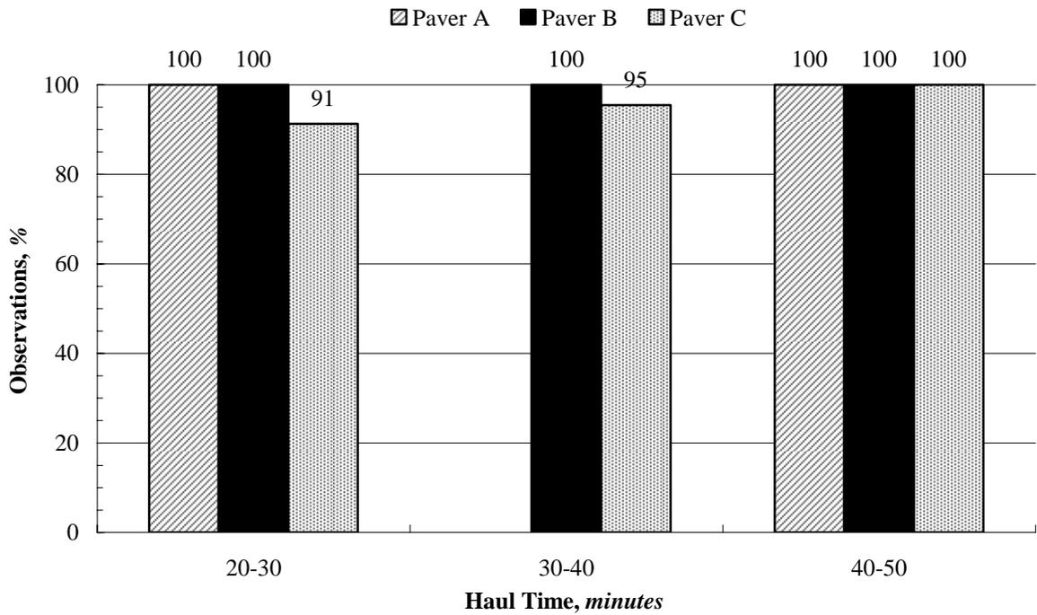
Figure B-4: TDD observations greater than one standard deviation from the mean located behind a paver.
