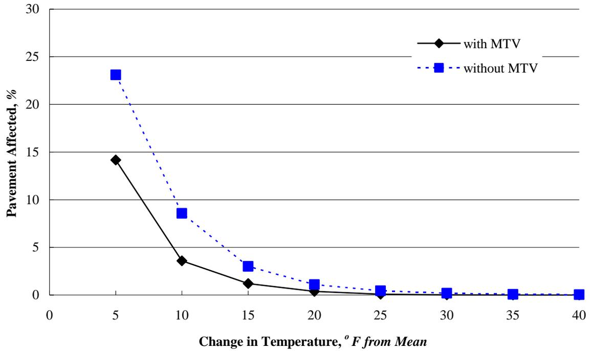
Figure 15: Effectiveness of material transfer vehicle (MTV) in reducing TDD (30–40 min. haul time).
