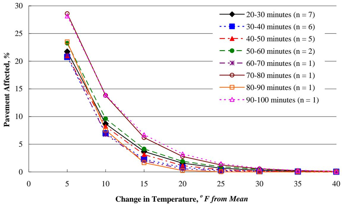
Figure 18: Effect of haul time on TDD.
