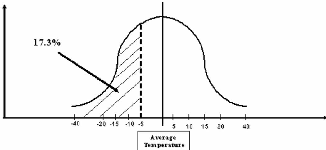
Figure 9: Typical curve used to calculate the percent of pavement affected by TDD.
