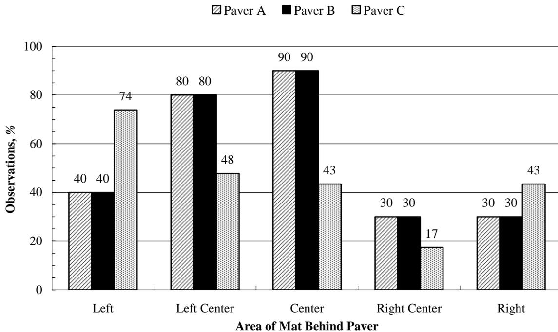
Figure B-6: TDD observations greater than one standard deviation from the mean in different locations behind the paver (20-30 min. haul time).
