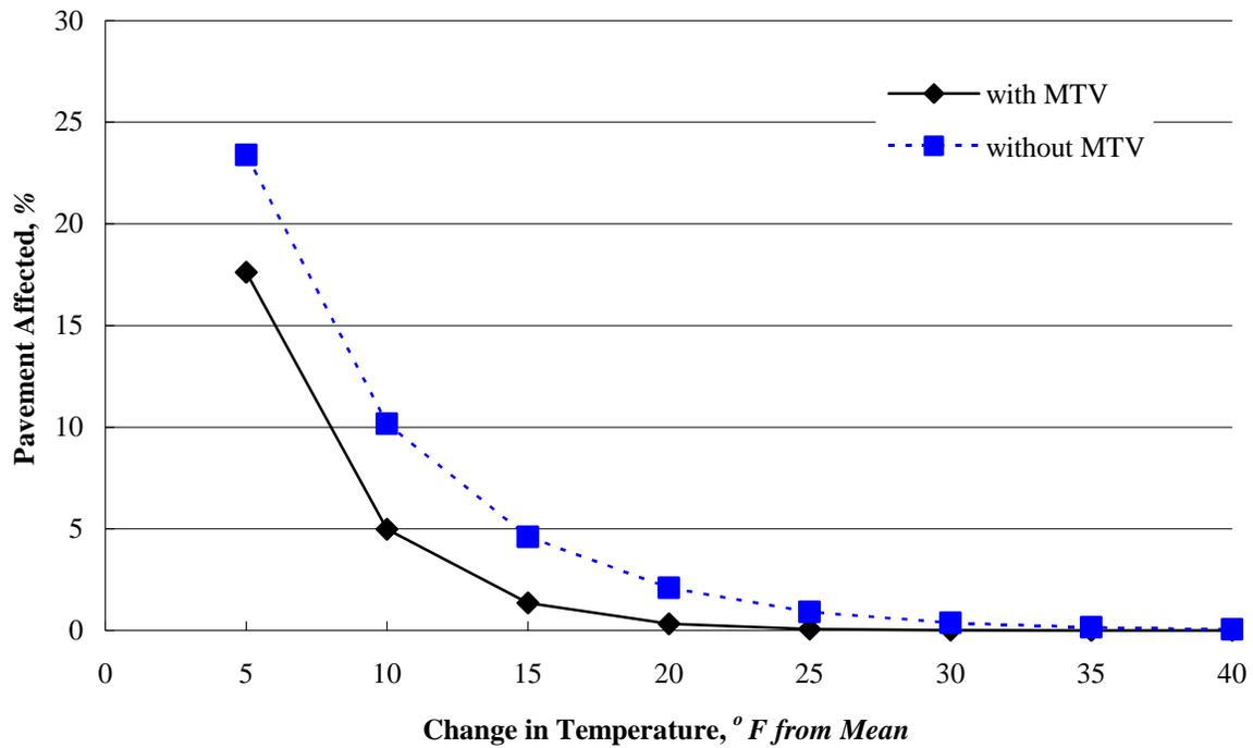
Figure 12: Effectiveness of material transfer vehicle (MTV) in reducing TDD (20–30 min. haul time).
