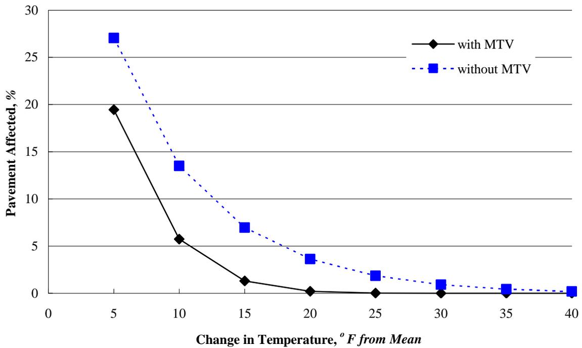
Figure 16: Effectiveness of material transfer vehicle (MTV) in reducing TDD (50–60 min. haul time).
