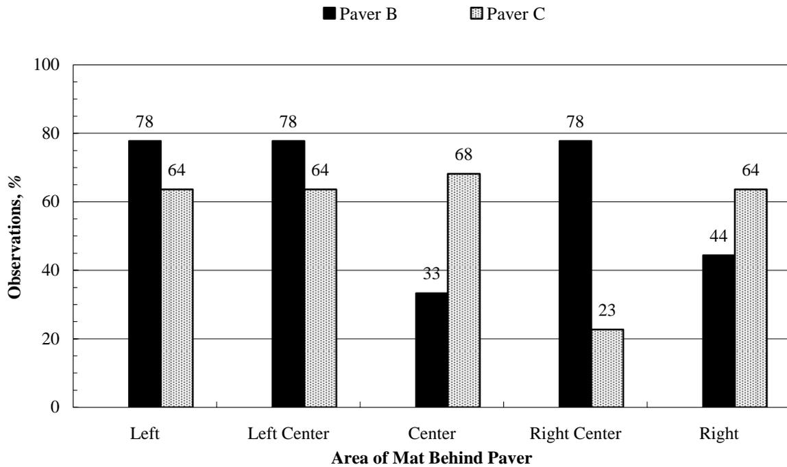
Figure B-8: TDD observations greater than one standard deviation from the mean in different locations behind the paver (30–40 min. haul time).
