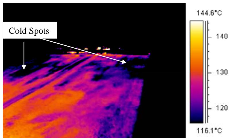
Figure 3: End of load temperature segregation.
