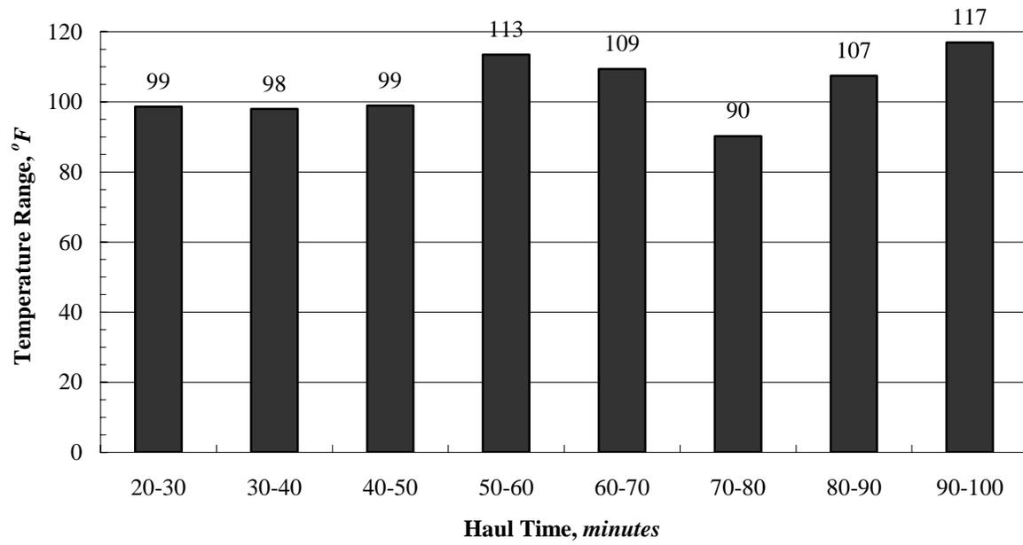
Figure B-13: Temperature range of HMA in trucks with respect to haul time.
