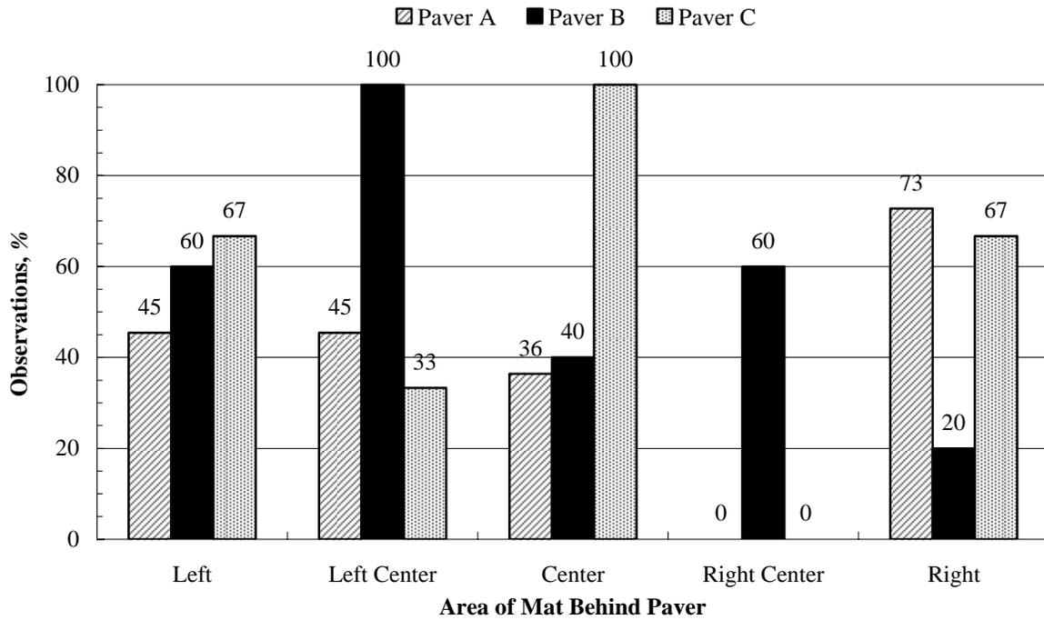
Figure B-10: TDD observations greater than one standard deviation from the mean in different locations behind the paver (40–50 min. haul time).
