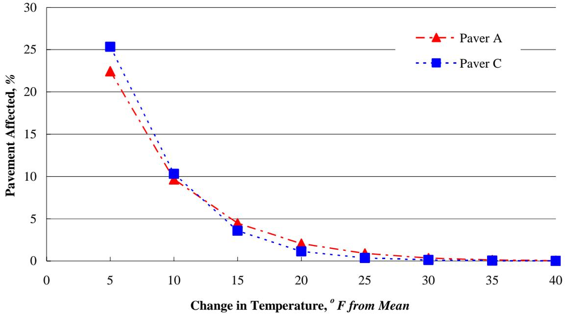
Figure B-3: Comparison of TDD from different asphalt pavers from different manufacturers (40–50 min. haul time, nighttime paving).
