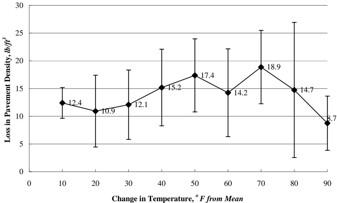
Figure 8: Effect of TDD on pavement density.
