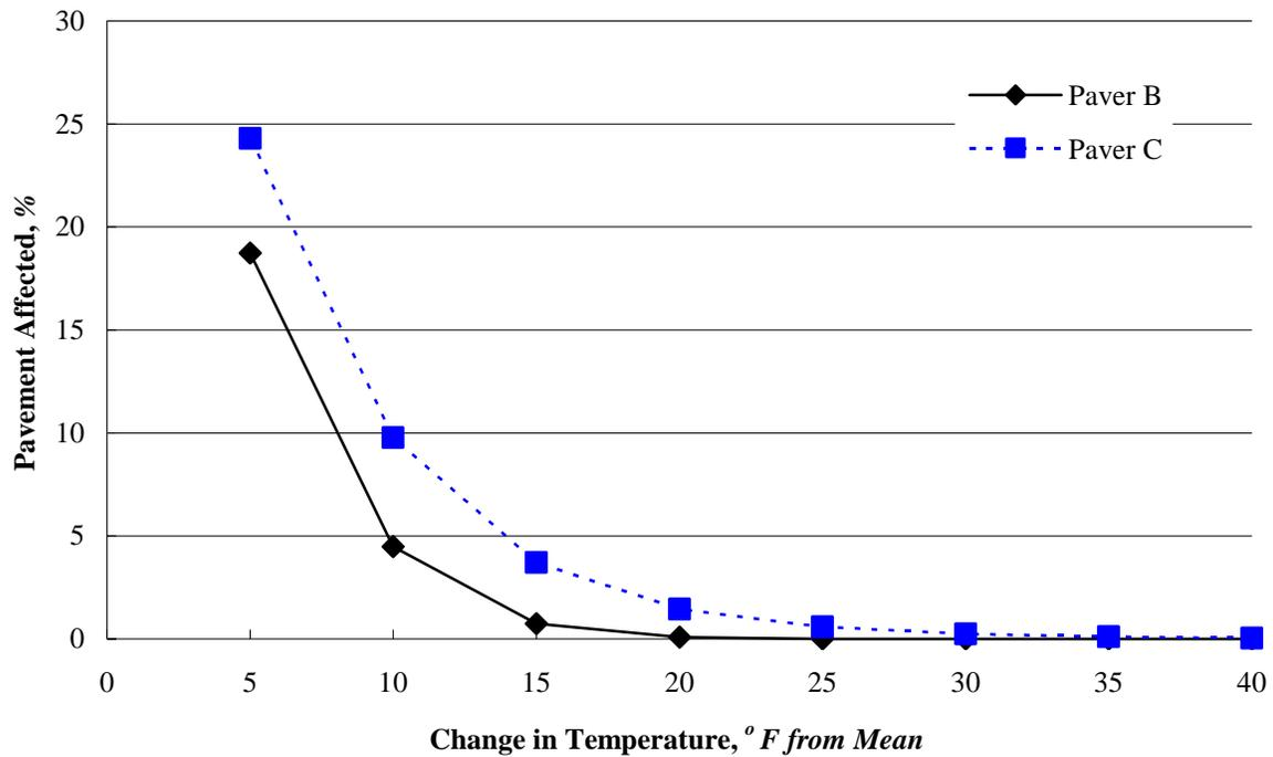
Figure B-1: Comparison of TDD from different asphalt pavers from different manufacturers (30–40 min. haul time).
