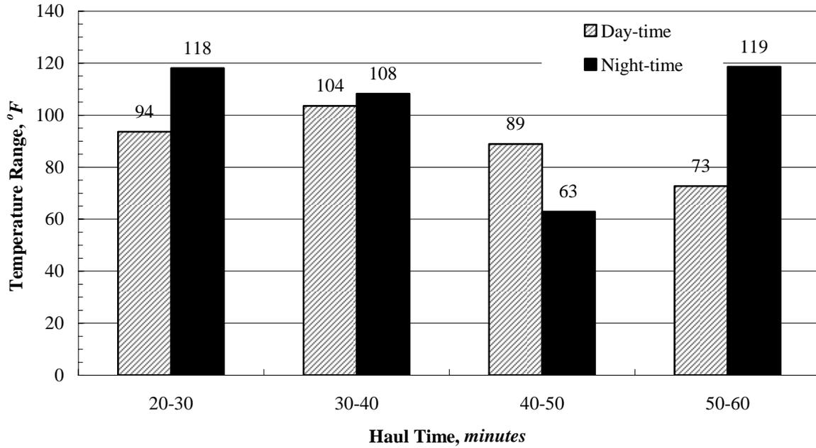
Figure 17: Temperature range of HMA in the truck bed.
