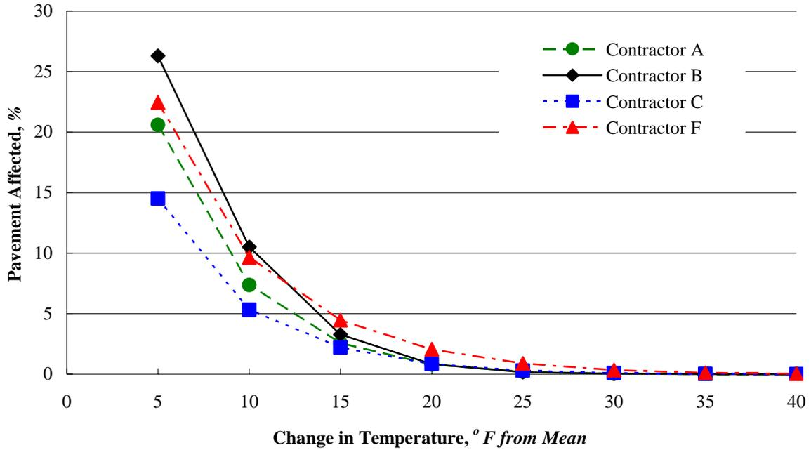
Figure 24: Effect of contractor on TDD (40–50 min. haul time).
