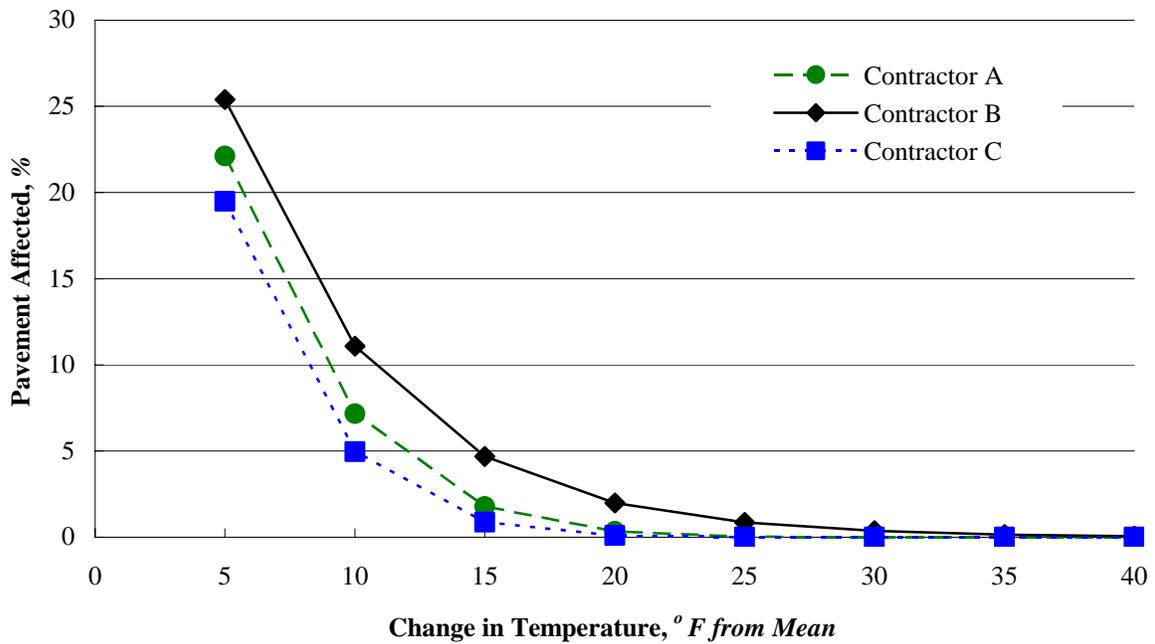
Figure 23: Effect of contractor on TDD (30–40 min. haul time).
