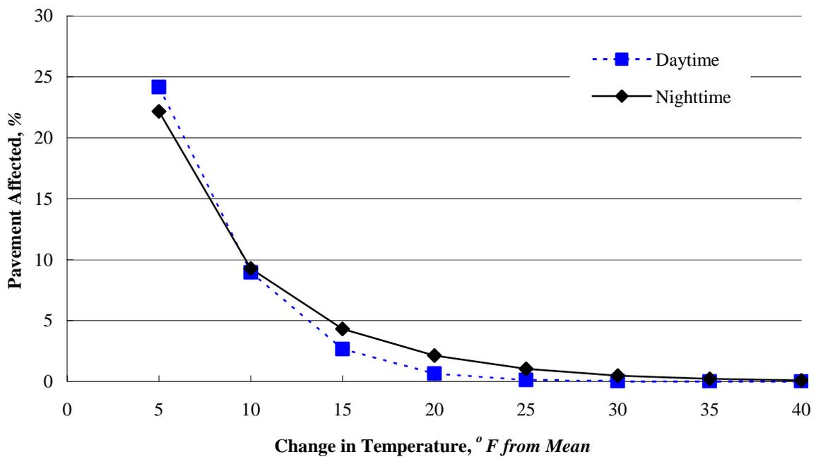
Figure B-12: Comparison of daytime vs. nighttime paving (20-30 min. haul time).
