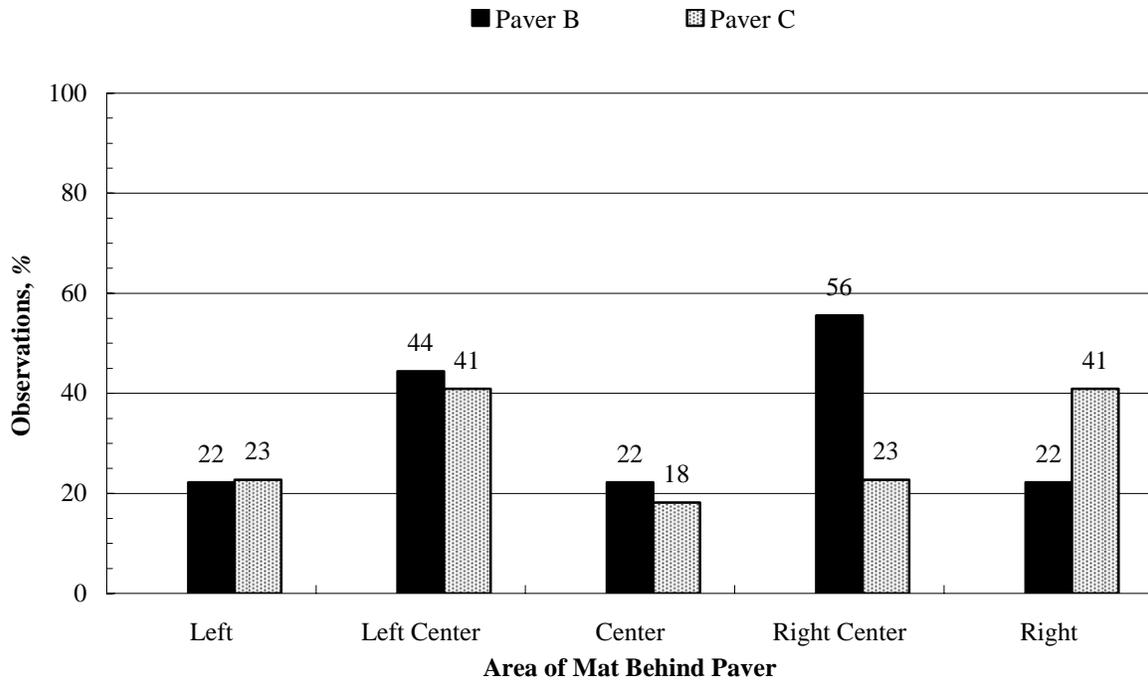
Figure B-9: TDD observations greater than two standard deviations from the mean in different locations behind the paver (30–40 min. haul time).
