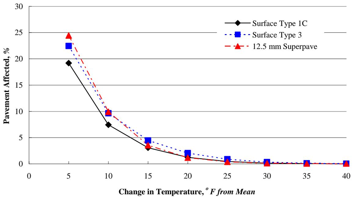
Figure 21: Effect of mix type on TDD (40–50 min. haul time).
